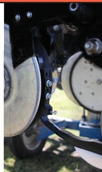
Fig. 13 While tightening final bolts pull back on Firmers to desired upright angle. Adjust the firmers and line up with the seed trench.
