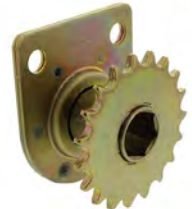
BEARING/SPROCKET Bearing with 19 tooth sprocket, 7/8" hex bore, 1-1/2" width. Used on John Deere 7200, 7300 and 1700 series planters row unit and planter drive line.
