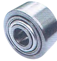
BEARING Closing wheel bearing for John Deere Model 7200, 7300 and IHC mode 296 & 386 planter, Bore Size: 0.669" round, O.D: 1.574" flat, IR width: 0.55", OR width : 0.472".
