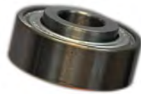
BEARING Ball bearing, ID: 15mm (.59"), OD: 42mm (1.65"), Width: 22mm (.87")
