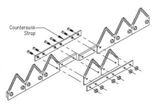
Remove 3 bolts (rivets) from ends of both sickle segments. Insert splice bolt through bottom countersunk strap, knifeback, section and top strap. Start nut on splice bolt with the triangular indents facing out. Hold head of bolt inside countersink in strap and tighten nut. NO ALLEN WRENCH NEEDED!
