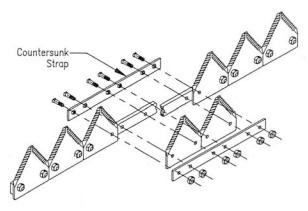
Remove 3 bolts (rivets) from one side of the break and 2 from the other side. One bolt will go through break. Insert splice bolt through bottom countersunk strap, knifeback section and top strap. Start nut on splice bolt with the triangular indents facing out. Hold head of bolt inside countersink in strap and tighten nut. NO ALLEN WRENCH NEEDED!
