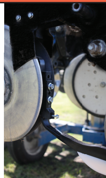
Fig. 13 While tightening final bolts pull back on Firmer to desired upright angle. Adjust the firmer and line up with the seed trench.
