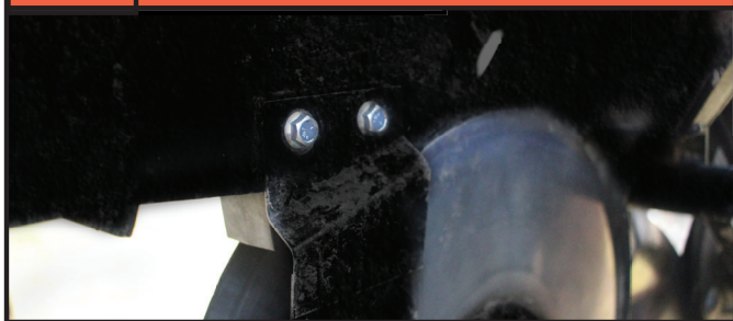
Fig. 12 Slide in the 2nd Spacer Tab on the opposite side. Place disk scrapper back into position and using the provided Bolts tighten to planter. Fig. 11 should allow for and easy install, but if you need more space: Loosen the bolts in Fig. 11
