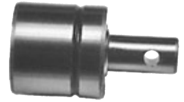
BEARING Bearing with cross hole to fit gauge wheel assemblies. Has a 40 mm O.D. to eliminate the use of the bearing spacer.
